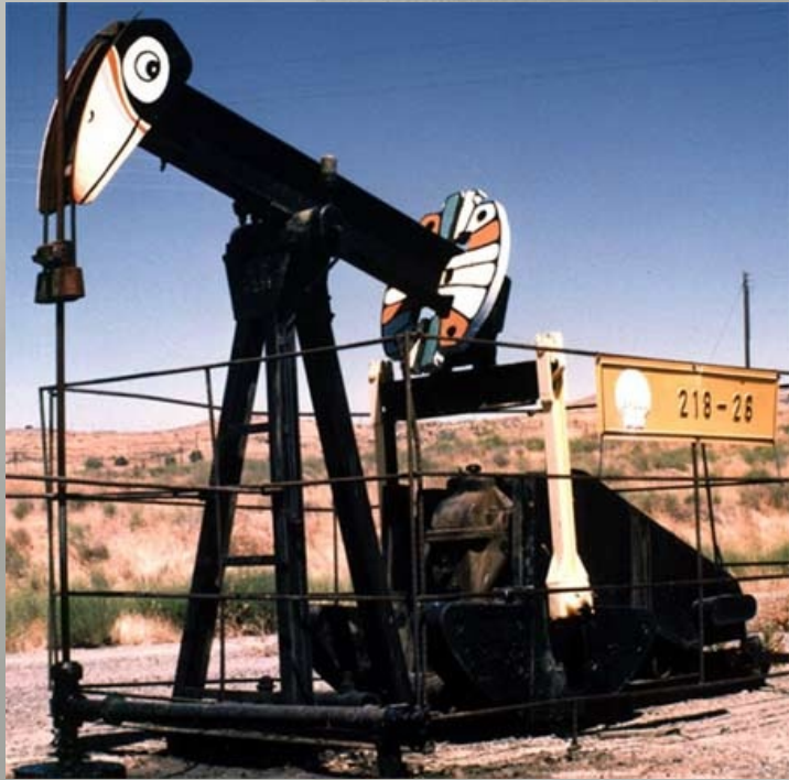
This “ nodding donkey ” is used to extract petroleum. Picture by US Dept. Energy.
