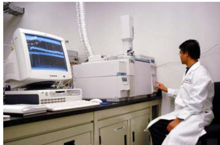
Environmental chemists frequently use [GC-MS](#) to analyze samples. The technique can detect very low concentrations of pollutants.
