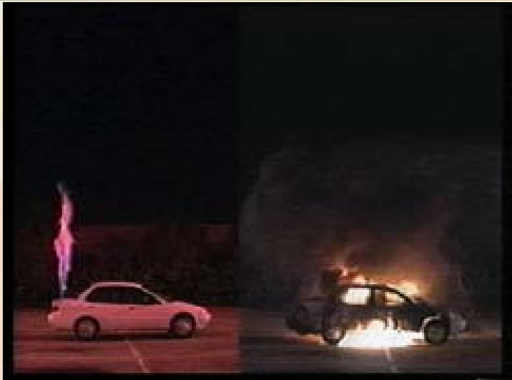
Photo 3 - Time: 1 min, 0 sec – Hydrogen flow is subsiding, view of gasoline vehicle begins to enlarge.
