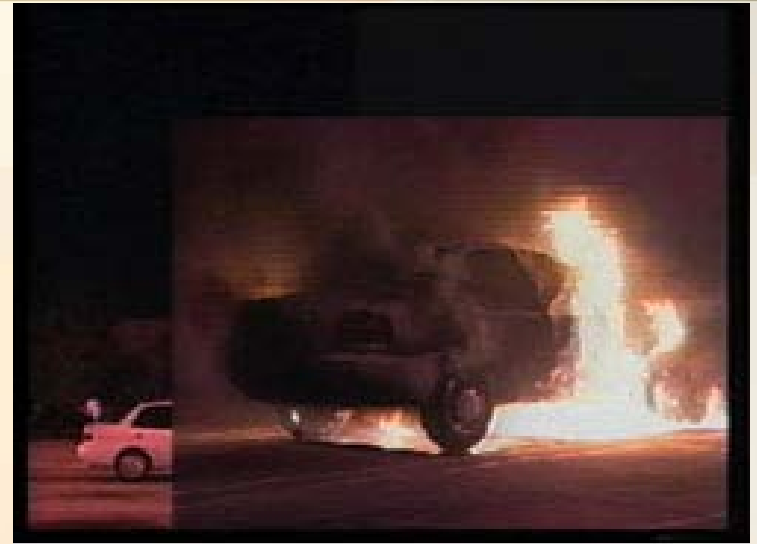
Photo 4 - Time: 1 min, 30 sec – Hydrogen flow almost finished. After this, the gasoline powered vehicle burns violently
